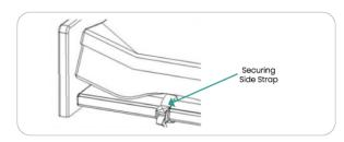
3. Secure the Control Unit at the foot end of the bed.
