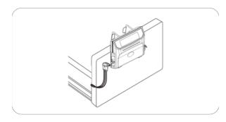
4. Remove the Protector Cap from the end of the air hose, and push the hose connector into the side of the Control Unit until you hear a 'click'. Connect the detection cable to the pump. To transport an inflated surface, first press 'Auto-Firm' for quick inflation, then cover the air hose with the Protector Cap - this keeps air in the surface for up to 24-hours.
